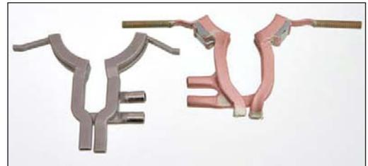
With GH microfusion technology, identical inductors can be produced from the same 3D manufacturing mold. This increases repeatability and consistency when multiple induction systems are running the same process, and significantly reduces maintenance and calibration time when inductors need to be changed out.
